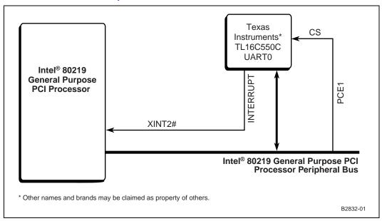
See datasheet at the following link for more information and a pin layout of this device: <a href="http://focus.ti.com/docs/prod/productfolder.jhtml?genericPartNumber=TL16C550C">http://focus.ti.com/docs/prod/productfolder.jhtml?genericPartNumber=TL16C550C</a>.
